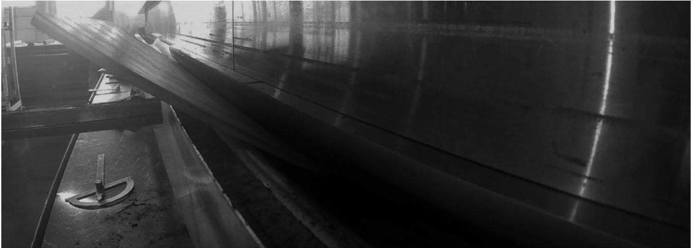
Swebor Armor™ 600 is an UHH protection steel which poses ability for cold forming. When cold forming Swebor Armor™ 600 personal safety precautions must be taken. We recommend bending of Swebor Armor™ 600 for the thickness.
